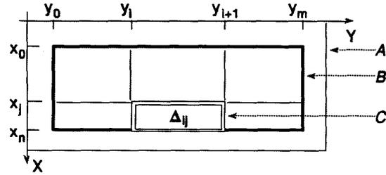
Figure 3: Fragmentation of field of vision into quasi-constant brightness zones  $\Delta_{ij}$ . Denotations: A — eye-sight, B — work space, C — splitting element
