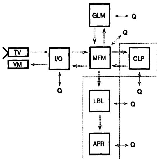
Figure 1: Architecture of the special video processor. Denotations: TV — TV camera; VM — video monitor; double arrows — data flows; dotted arrows — analog video dates; single arrows — system bus links; I/O — input/output module; MFM — multifunctional module; GLM — gray level memory module; CLP — "cell logic processor" module; LBL — "Label" module; APR — "Arithmetical processor" module; dotted rectangles — optional elements.
